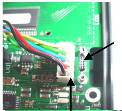
Shunt Calibration Resistor
