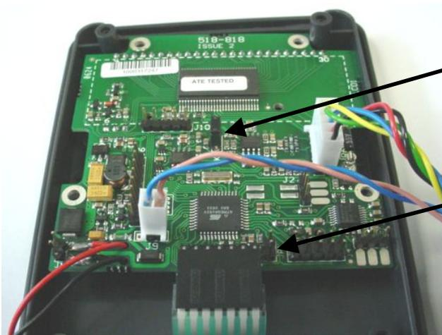
Sensitivity link should be in this position for use with sensors, with sensitivities <math>\lt; \pm 5\text{mV/V}</math>
