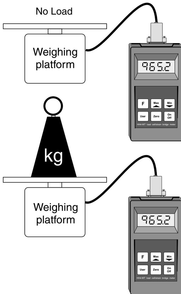
Perform **CAL 1** and **SCL 1** operation with no load or low load.
