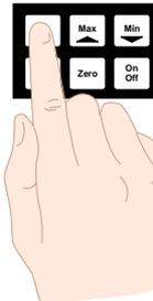
1. Switch on the instrument. When the "wake up" messages have finished and the display has settled down to its normal reading press then release the **F** button.
