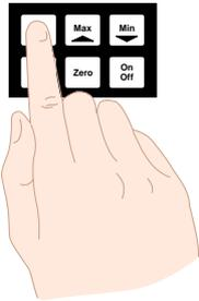
1. Switch off the instrument. Hold in the **F** button and switch on. The display will indicate **CAL** as part of the "wake up messages" when the **CAL** message is seen you can release the button.
