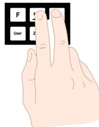
2. Within 2 seconds of releasing the **F** button press then release the **▲** and **▼** buttons together. The display will now indicate **FUNC** followed by the first function.
